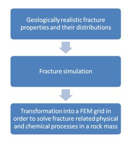
*Figure 3. The use of geologically realistic fracture patterns in fracture simulation, in groundwater modelling and in estimating heat transfer in a rock mass.*
